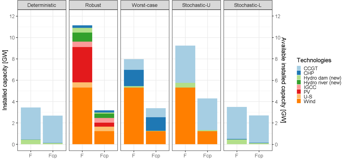
Figure 1: Electricity capacity mix (Full capacity F and available capacity Fcp ) for the five investment strategies: Deterministic , Robust , Worst-case , Stochastic-U and Stochastic-L . (Acronyms: Photovoltaics (PV), Combined Cycle Gas Turbine (CCGT), Cogeneration of Heat and Power (CHP), Integrated Coal Gasification Combined Cycle (IGCC), Ultra-Supercritical Coal (U-S))
